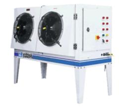
Group fitted with body envisaged for installation with external with built-in electrical equipment box, Hermetic Compressor 1 cv equipped with integral protection, Resistance of pre-heating of the compressor, Ventilators high-output helicoid condensers and low noise level, Control of the pressure of condensation with pressure controller, Pressostats high and low pressure, Voyant of liquid, tank of liquid with R404A.
