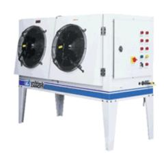
Group fitted with body envisaged for installation with external with built-in electrical equipment box, Hermetic Compressor 1.2 cv equipped with integral protection, Resistance of pre-heating of the compressor, Ventilators high-output helicoid condensers and low noise level, Control of the pressure of condensation with pressure controller, Pressostats high and low pressure, Voyant of liquid, tank of liquid with R404A.
