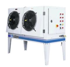
Group fitted with body envisaged for installation with external with built-in electrical equipment box, Hermetic Compressor 2 cv equipped with integral protection, Resistance of pre-heating of the compressor, Ventilators high-output helicoid condensers and low noise level, Control of the pressure of condensation with pressure controller, Pressostats high and low pressure, Voyant of liquid, tank of liquid with R404A.
