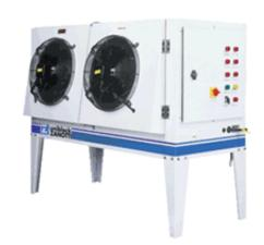
Group fitted with body envisaged for installation with external with built-in electrical equipment box, Hermetic Compressor 3 cv equipped with integral protection, Resistance of pre-heating of the compressor, Ventilators high-output helicoid condensers and low noise level, Control of the pressure of condensation with pressure controller, Pressostats high and low pressure, Voyant of liquid, tank of liquid with R404A.
