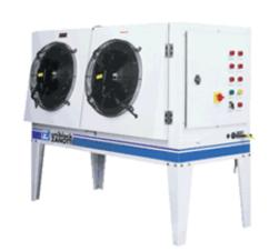
Group fitted with body envisaged for installation with external with built-in electrical equipment box, Hermetic Compressor 4 cv equipped with integral protection, Resistance of pre-heating of the compressor, Ventilators high-output helicoid condensers and low noise level, Control of the pressure of condensation with pressure controller, Pressostats high and low pressure, Voyant of liquid, tank of liquid with R404A.
