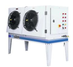
Group fitted with body envisaged for installation with external with built-in electrical equipment box, Hermetic Compressor 5 cv equipped with integral protection, Resistance of pre-heating of the compressor, Ventilators high-output helicoid condensers and low noise level, Control of the pressure of condensation with pressure controller, Pressostats high and low pressure, Voyant of liquid, tank of liquid with R404A.
