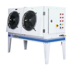
Group fitted with body envisaged for installation with external with built-in electrical equipment box, Hermetic Compressor 7.5 cv equipped with integral protection, Resistance of pre-heating of the compressor, Ventilators high-output helicoid condensers and low noise level, Control of the pressure of condensation with pressure controller, Pressostats high and low pressure, Voyant of liquid, tank of liquid with R404A.
