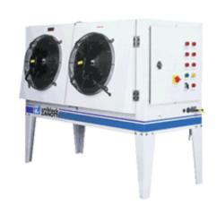
Group fitted with body envisaged for installation with external with built-in electrical equipment box, Hermetic Compressor 10 cv equipped with integral protection, Resistance of pre-heating of the compressor, Ventilators high-output helicoid condensers and low noise level, Control of the pressure of condensation with pressure controller, Pressostats high and low pressure, Voyant of liquid, tank of liquid with R404A.
