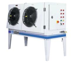
Group fitted with body envisaged for installation with external with built-in electrical equipment box, Hermetic Compressor 15 cv equipped with integral protection, Resistance of pre-heating of the compressor, Ventilators high-output helicoid condensers and low noise level, Control of the pressure of condensation with pressure controller, Pressostats high and low pressure, Voyant of liquid, tank of liquid with R404A.
