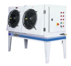
Group fitted with body envisaged for installation with external with built-in electrical equipment box, Semi hermetic Compressor 35 cv equipped with integral protection, Resistance of pre-heating of the compressor, Ventilators high-output helicoid condensers and low noise level, Control of the pressure of condensation with pressure controller, Pressostats high and low pressure, Voyant of liquid, tank of liquid with R404A.
