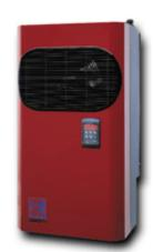
Monobloc with wall fitted with body with integrated electrical equipment box, cast solid Evaporator, panel of regulation integrated Compressing hermetic 3/8 cv equipped with integrale protection Expansion of gas by capillaire
